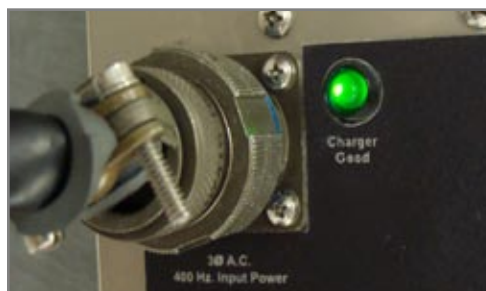
Figure 3.9.3 - “Charger Good” LED
