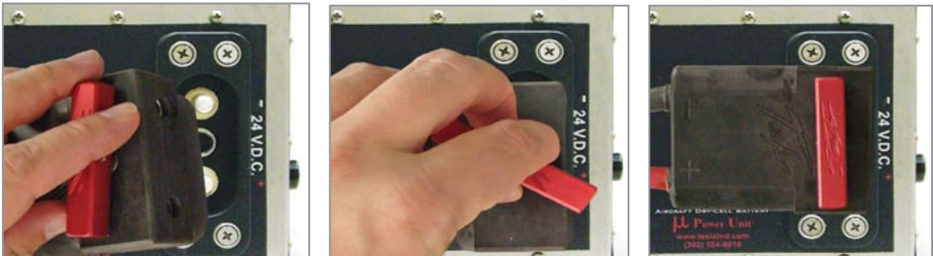
Figure 3.11.1 Attaching DC Power Cable to TIAH64D MPU-24
