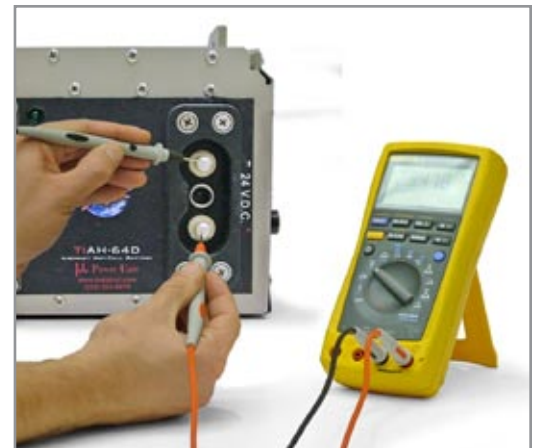
Figure 5.2.3 – Testing DC Receptacle
