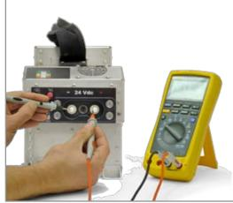
Figure 3.9.3 – Testing DC Receptacle
