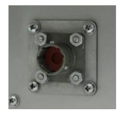
Figure 2.12.3 -**TI2000-271** Dummy Receptacle installed on the TI58D-R17 MUP-24
