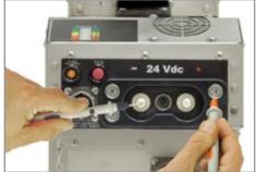
**5.** Move the negative probe to the dc negative post on the dc output connector.
