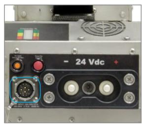
Figure 3.12.1 AC Input Connector (outlined in blue)
