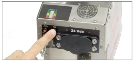
Figure 2.8.1 "Press for Capacity" button
