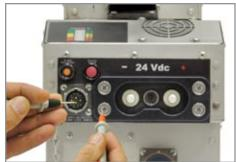
**4.** Move the positive probe to one of the four screws securing the dc output connector to the unit casing.
