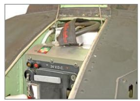
Figure 2.10.2 - Battery Compartment
