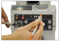
Place the negative probe on the ac ground probe (J or L) and the positive probe on an exposed part of the metal case.
