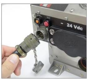
Figure 3.12.2 Attaching AC Line Cord
