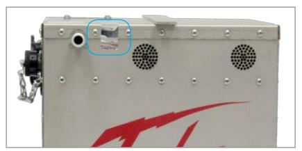
Figure 6.3.1 - Warranty Void stickers on the TI47UH1 MPU-24
