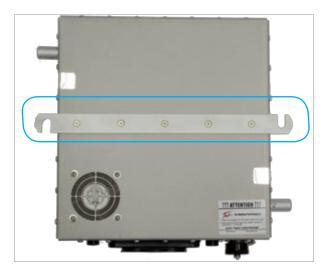
Figure 3.8.1 – Battery Lock-down (outlined in blue)
