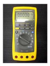
Figure 4.9.1 – Digital Multimeter
