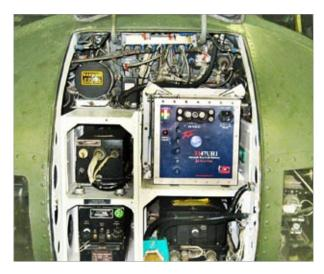
Figure 3.9.1 –TI47UH1 properly installed in a UH-1 Huey (DC Plug is not secured)
