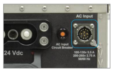
Figure 3.6.1 AC Input Connector (outlined in blue)
