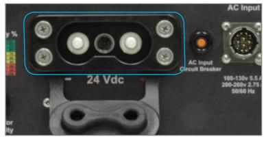
Figure 3.2.1 DC Output Connector (outlined in blue)
