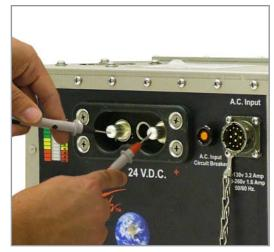
Figure 4.9.3 - Testing DC Receptacle
