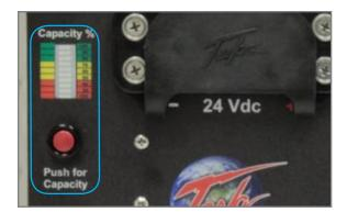
Figure 3.7.1 "Press for Capacity" button location (outlined in blue)
