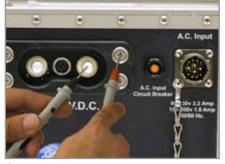
Move the negative probe to the dc positive post on the DC Output Connector.
