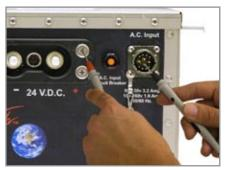
**4.** Move the positive probe to one of the four screws securing the DC Output Connector to the unit casing.
