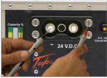
**5.** Move the negative probe to the dc negative post on the DC Output Connector.
