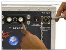
Move the positive probe to the dc positive post on the DC Output Connector.
