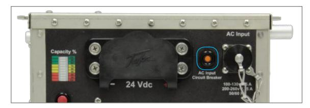
Figure 3.4.1 AC Input Circuit Breaker location (outlined in blue)
