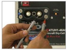
**6.** Move the negative probe to the dc positive post on the DC Output Connector.
