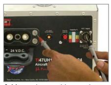
4. Move the positive probe to one of the four screws securing the DC Output Connector to the unit casing.
