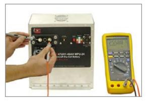
Figure 4.9.3 - Testing DC Receptacle
