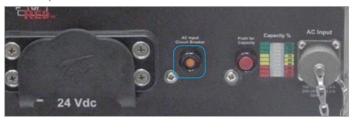
Figure 3.2.1 AC Input Circuit Breaker location (outlined in blue)
