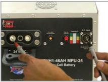
**3.** Move the positive probe to the dc negative post on the DC Output Connector.
