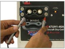
**5.** Move the negative probe to the dc negative post on the DC Output Connector.
