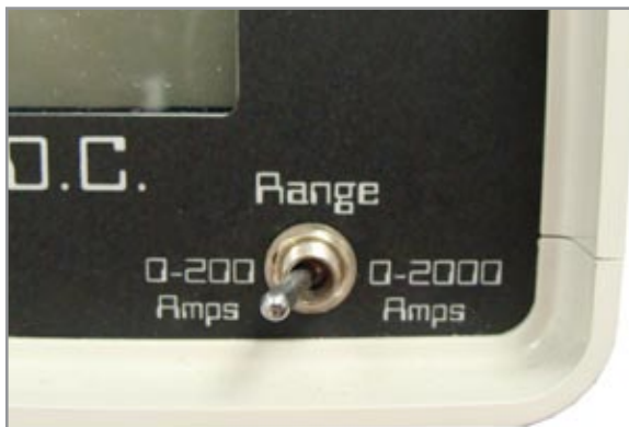
2.3.1 - Switched to 0-200 Amps
