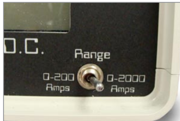
2.3.2 - Switched to 0-2000 Amps
