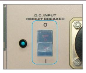
Figure 2.12.1 - DC Input Circuit Breaker (outlined in blue)
