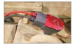
Figure 3.7.1 Attaching DC Power Cable to ground vehicle
