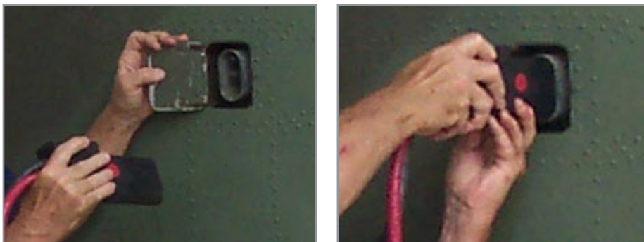
Figure 3.7.3 Attaching DC Power Cable to aircraft
