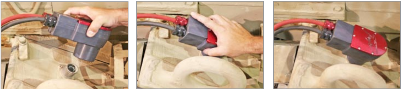
Figure 3.7.2 Attaching DC Power Cable to ground vehicle
