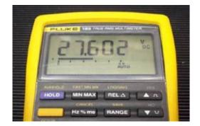
Figure 6.2.5 – Multimeter reading typical 24 V power cell voltage
