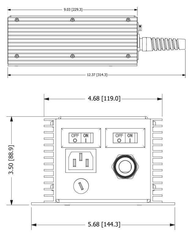
*Measurements are in inches and millimeters* Figure 2.4.1 – TI150 Battery Charger/Conditioner Physical Dimensions
