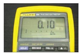
Figure 6.2.2 – Multimeter reading continuity
