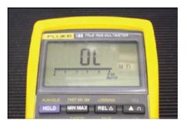
Figure 6.2.3 – Multimeter reading open circuit
