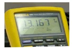
Figure 6.2.4 – Multimeter reading typical 12 V power cell voltage
