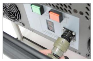
Figure 3.16.2 Connecting DVAM to Interface Receptacle
