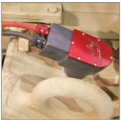
Figure 3.13.2 Attaching NATO DC Power Cable to vehicle
