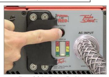
Figure 2.8.1 - "Push to Test" button
