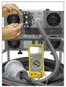
Figure 3.9.2 - Testing DC Receptacle
