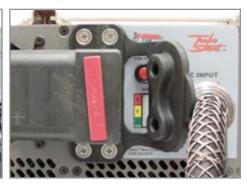
Figure 3.13.1 Attaching DC Power Cable to unit
