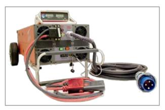
Figure 3.16.3 DVAM and cables connected to GPU
