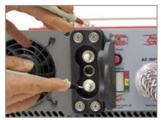
1. Place the negative probe on the ac ground probe and the positive probe on the case.
