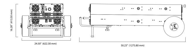
Figure 2.5.1 - TI5400 GPU-24 physical dimensions
