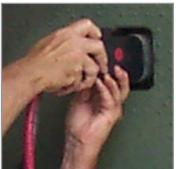
Figure 3.13.3 Attaching an Aviation DC Power Cable to aircraft
