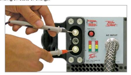
Figure 3.8.3 - Testing DC Receptacle
