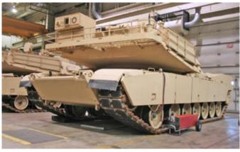
Figure 3.11.3 Starting vehicle with TI5200 GPU-24
