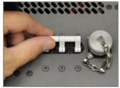
Figure 3.16.6 Switching Circuit Breaker ON
