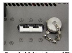
Figure 3.16.5 Circuit Breaker OFF
