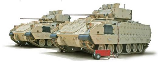
Figure 3.11.3 Starting vehicle with TI5100 GPU-24
