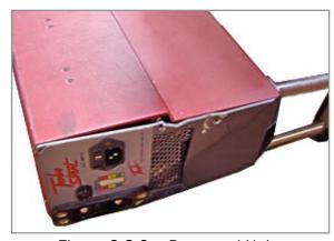
Figure 3.8.2 – Damaged Unit Misaligned Case with Bent Faceplate
