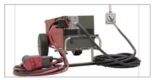
Figure 3.13.2 Connecting TI5100 GPU-24 to AC Power Supply with DC Power Cable Attached
