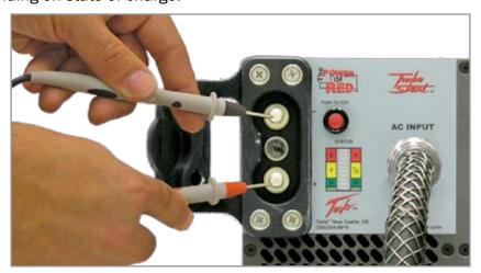
Figure 3.8.3 – Testing DC Receptacle
