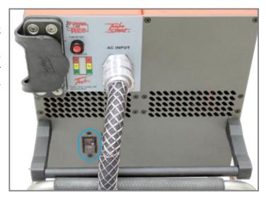
Figure 3.15.1 Circuit Breaker Selector Switch (outlined in blue)
