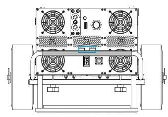
Figure 2.11.1 - Location of the DC Output On and Off Buttons (outlined in blue)
