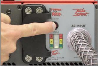
Figure 2.8.1 - "Push to Test" button
