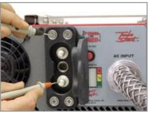
2. Move the positive probe to the dc positive post.
