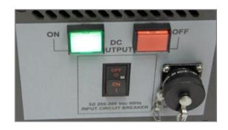
Figure 2.11.2 - DC Output "On" and "Off" Buttons
