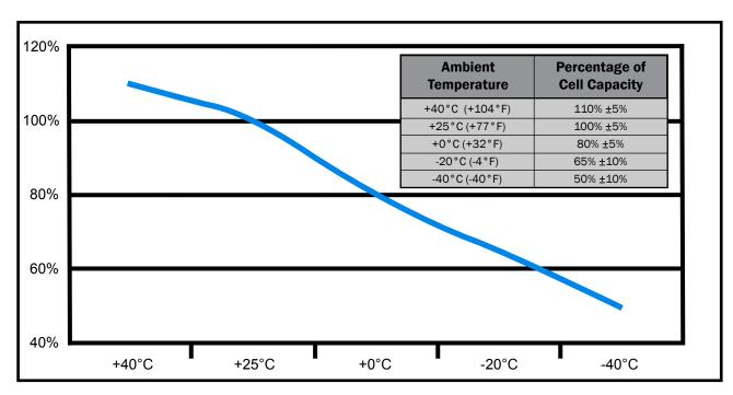
Figure 3.6.1 – Output power capability versus ambient temperature
