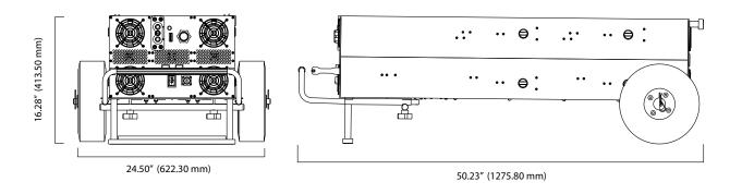
Figure 2.5.1 - TI4400 GPU-24 physical dimensions
