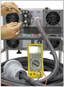
Figure 3.9.2 – Testing DC Receptacle
