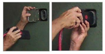
Figure 3.13.3 Attaching an Aviation DC Power Cable to aircraft
