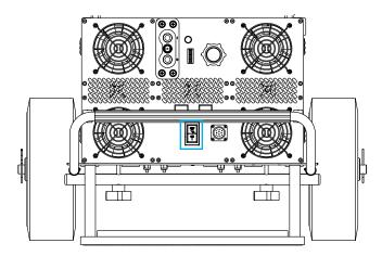
Figure 2.9.1 - Location of the 60Hz 3-Phase AC Input Circuit Breaker (outlined in blue)
