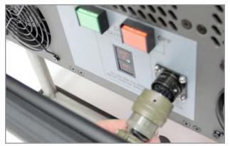
Figure 3.16.2 Connecting DVAM to Interface Receptacle
