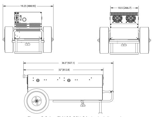
Figure 3.2.1 – TI4100 GPU-24 physical dimensions
