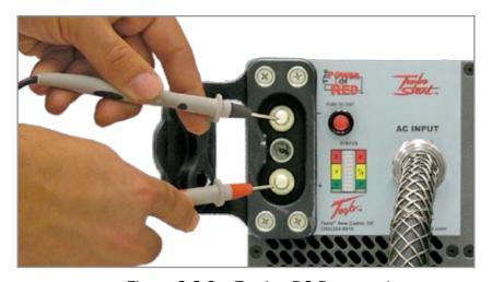
Figure 3.8.3 – Testing DC Receptacle
