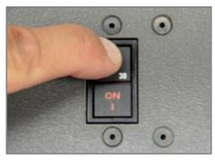
Figure 3.16.2 Switching Circuit Breaker OFF
