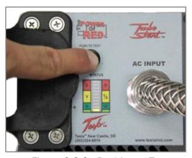
Figure 2.8.2 - Pushing to Test
