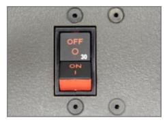
Figure 3.16.3 Circuit Breaker OFF
