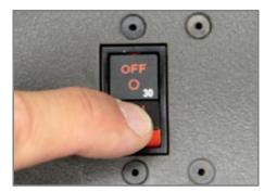
Figure 3.16.6 Switching Circuit Breaker ON
