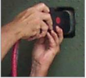
Figure 3.11.3 Attaching an Aviation DC Power Cable to aircraft
