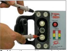
**2.** Move the positive probe to the dc positive post.
