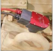
Figure 3.11.2 Attaching NATO DC Power Cable to vehicle
