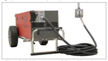
Figure 3.16.4 Plugging Into AC Single Phase Power
