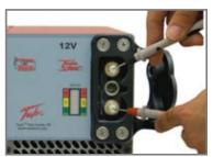
3.8.8 - Measuring Voltage on DC Output Connector
