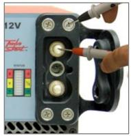
3.8.4 - DC Output Connector Positive Pin
