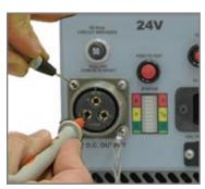
3.8.7 - DC Output Connector Positive Pin
