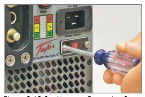
Figure 2.13.2 - Unscrew Protective Cover
