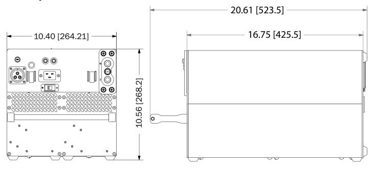
Figure 2.5.1 – TI1550 12-24-UAV GPU physical dimensions
