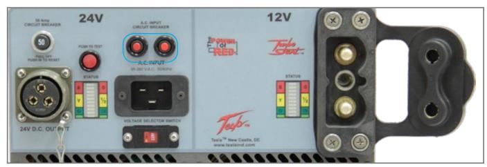
Figure 2.8.1 - AC Input Circuit Breaker (outlined in blue)
