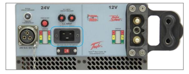
Figure 2.9.1 - AC Input Connector (outlined in blue)
