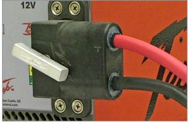
Figure 3.11.1 Attaching DC Power Cable to GPU
