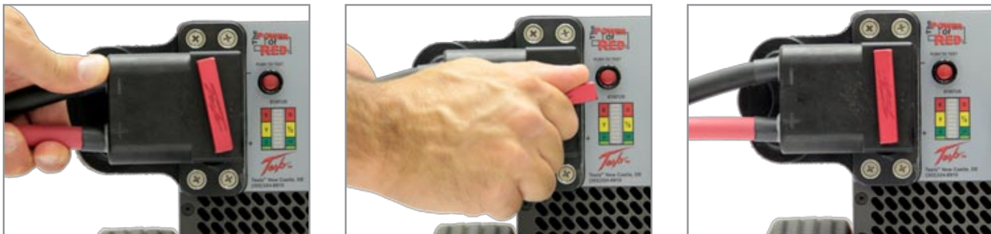
Figure 3.11.1 Attaching DC Power Cable to TI1500 GPU-12
