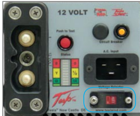
Figure 2.10.1 Input Voltage Selector Switch (outlined in blue)
