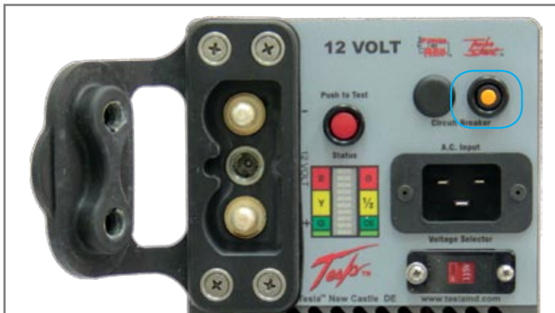
Figure 2.8.1 - AC Input Circuit Breaker (outlined in blue)
