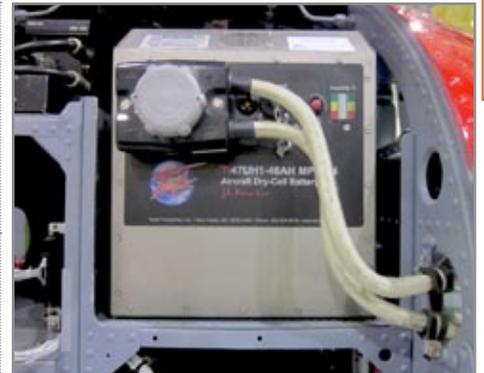
Designed to fit the Cal Fire UH1 Huey Helicopter.
