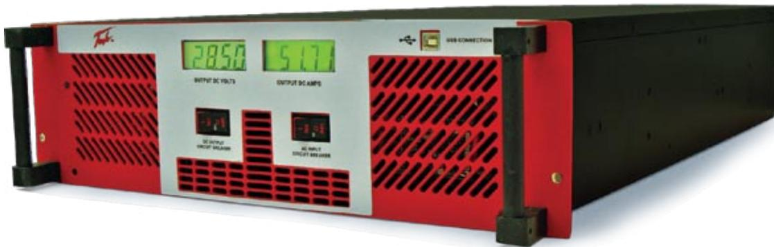
The Tesla™ Astrapi i Rack Mount Power Supply Module is expertly engineered as a single source of clean power for data centers and industrial control and communication equipment. The Power Supply Module is capable of delivering 6.3 kVA of reliable, filtered, regulated DC power while operating from single-phase ac power. As always, the unit is backed by a Tesla™ 2-year warranty, a trained support team, and an experienced staff of customer service professionals.
